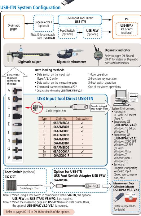
The input tool is automatically recognized as an HID\* keyboard device (a standard Windows driver) just by connecting it to a USB port.
